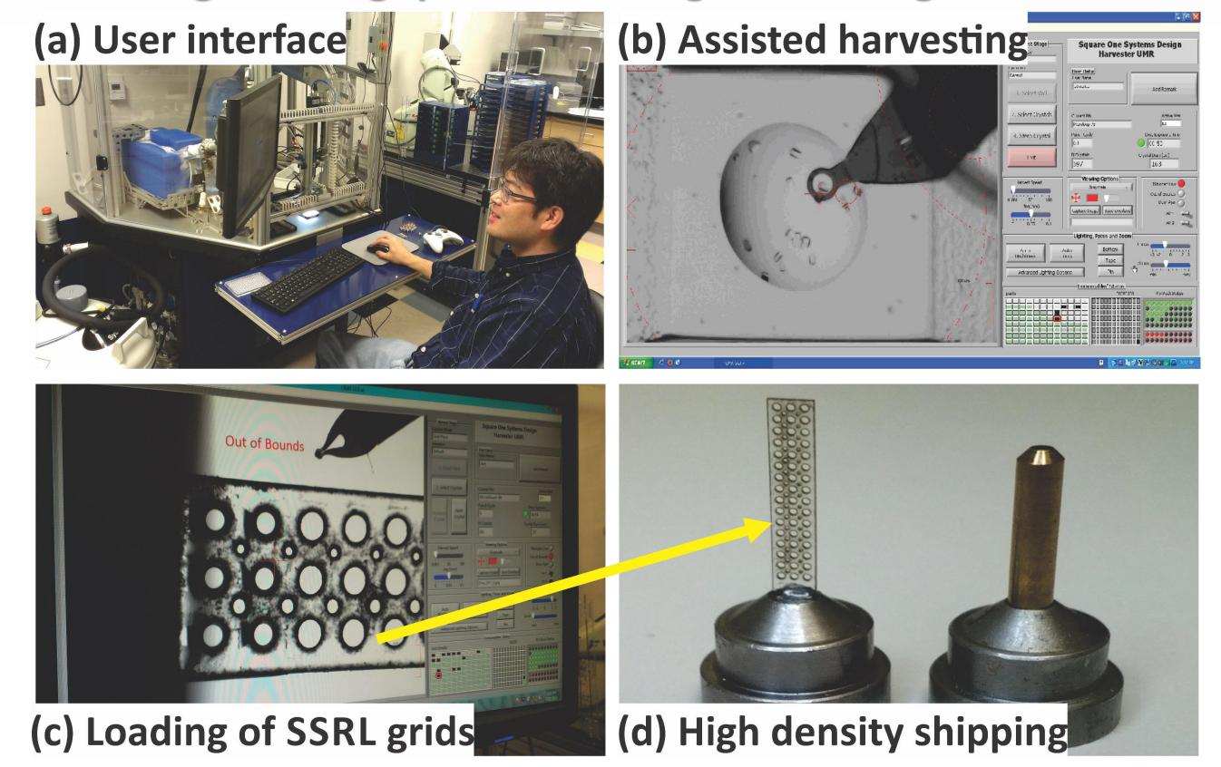
(a)  $\rightarrow$  (d) Workflow of robot-assisted harvesting into SSRL sample mounting grids. UMR represents an opportunity for high-density shipping to FEL sources.
