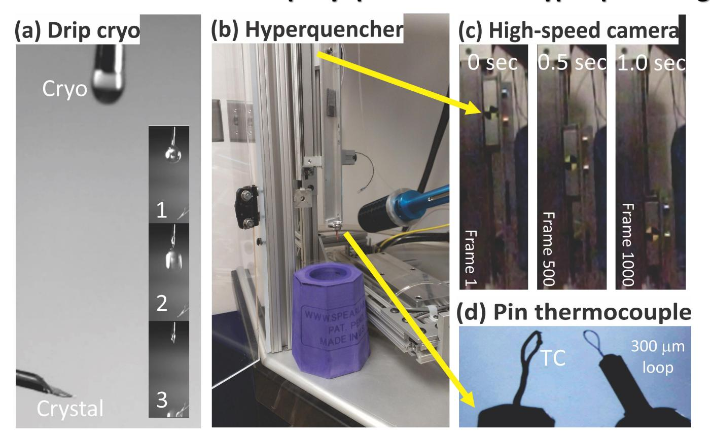
(a) Automated drip cryo mechanism for harvested crystals provides insulation from film boiling regime of liquid nitrogen (PFO oil). (b) Directly coupled pneumatic hyperquencher cools crystals at high-speed (5 m/s) in nucleate boiling regime of liquid nitrogen. (c) High-speed camera (1000 frames/s) allows accurate calculation of hyperquencher speeds. (d) High-rate data acquisition thermocouple allows for precise monitoring of cooling rates.
